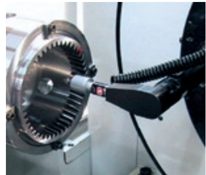
Integrated measuring of internal workpieces
