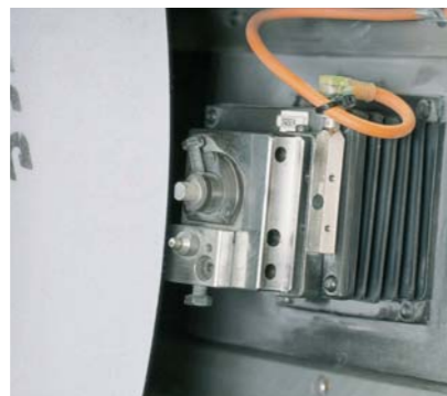
Dressing unit with diamond for rough and finish dressing
