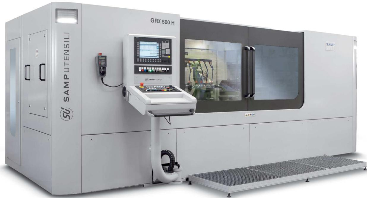
The GRX 500 H is a larger version of the GR, thanks to the presence of the on-board dressing wheel. The machine is suitable for the manufacture of very large screws and rotors. In addition, the machine mounts an additional NC axis, allowing you to work with two grinding wheels.
