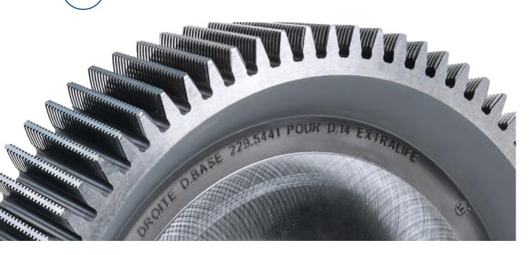
Since many years, shaving is known as a big batch production gear finishing process in the automotive and truck industry.
