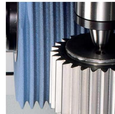
Universal quick change clamping systems for mass production environments allow rapid tool change so valuable grinding time is never compromised.
