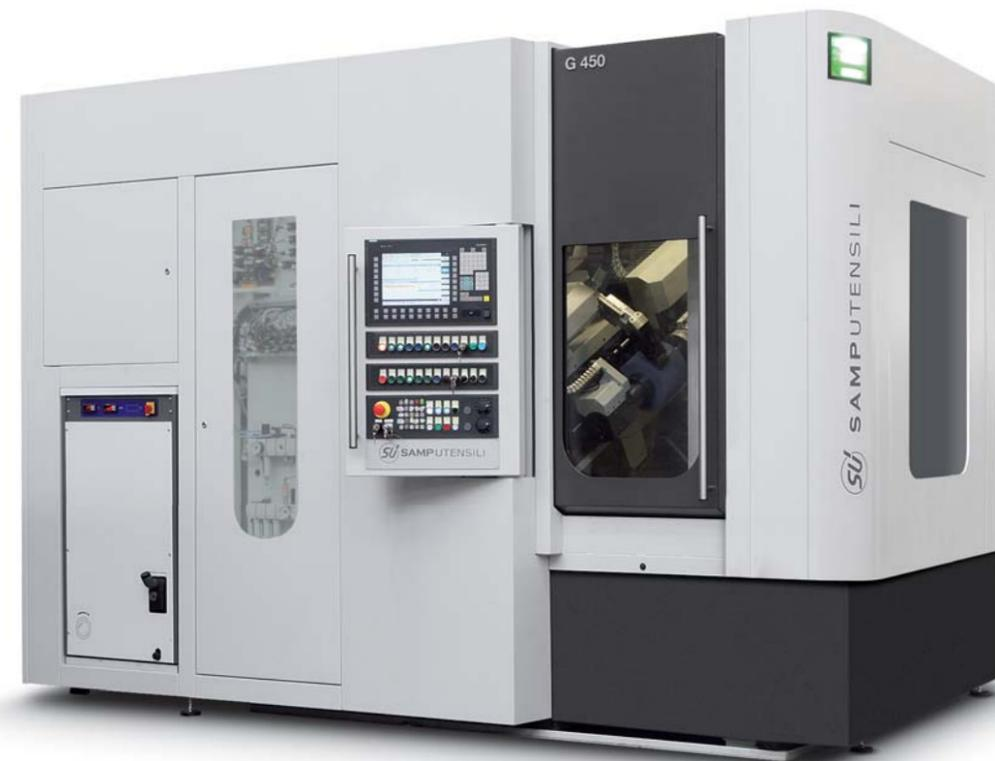
The Samputensili G 250 / G 450 is a machine platform, available in two sizes, based on established concepts of the best-selling Samputensili S 250/400 G machine, which have been further enhanced and improved. The result is an innovative, compact and extremely flexible gear grinding machine.
