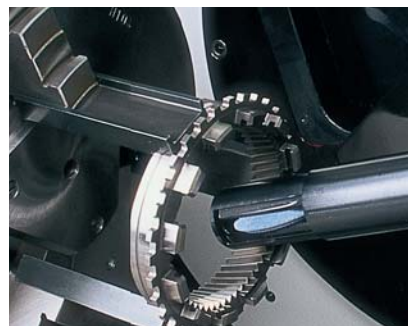
Grinding of helical internal gear
