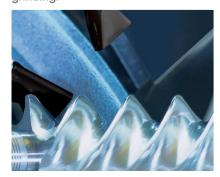
Optionally it is also possible to grind spur or helical internal gears.
