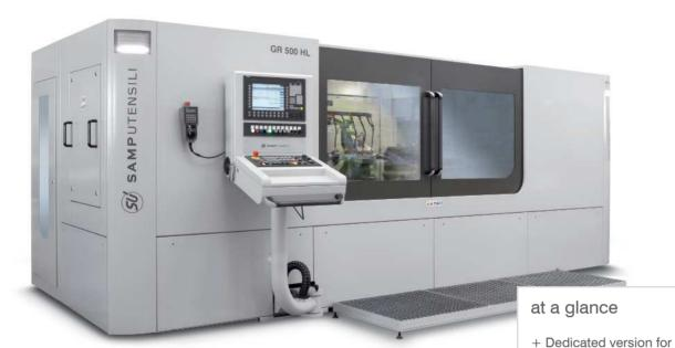
The GR 500 HL has been specifically designed for efficient high precision grinding of a wide range of screw-type profiles including worms, ball screws, rotors, hydraulic pump screw.
