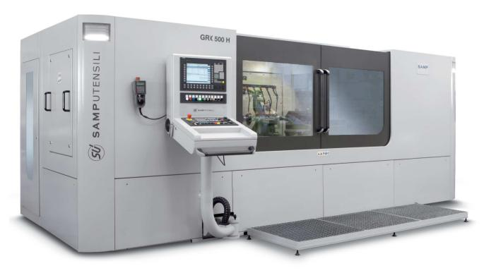
The GRX 500 H is a larger version of the GR, thanks to the presence of the onboard dressing wheel. The machine is suitable for the manufacture of very large screws and rotors. In addition, the machine mounts an additional NC axis, allowing you to work with two grinding wheels.
