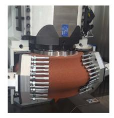
or two CBN electroplated grinding wheels. These two possible set-up make the GW3600HD the perfect solution both for the prototyping and for the mass production.
