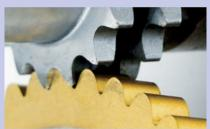
Rolling of a chain sprocket gear
