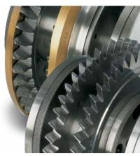
Back: Monoblock chamfering and deburring solution on one tool head Front: set of rolling tools on one tool head
