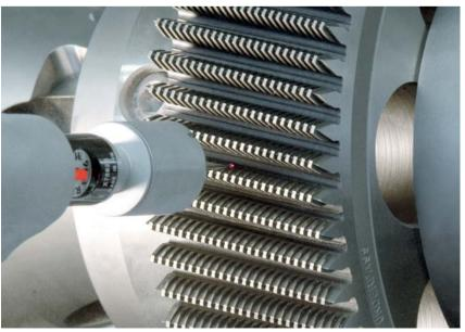
Sharpening and in-machine measurement of shaving cutters
