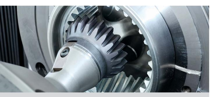
Star SU and Profilator have formed an alliance to manufacture Scudding® tools for the global market. Scudding® is a continual gear cutting process which makes both the production of external and internal gears, as well as spur and helical gearing possible.
