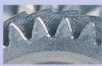
Workpiece after chamfering and deburring
