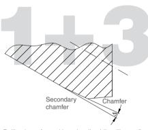
Rolling is performed by a localized "levelling out" action which may be described as a second chamfer with a chamfering angle  $\Delta$  of about 1°.
